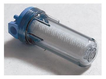
The wound process produces the formation of thousands of channels with a controlled porosity decreasing from the outside section to the inner layer. Progressive removal of particles provides true depth filtration and high dirt holding capacity.
